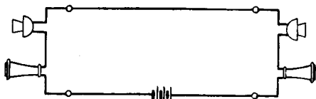
FIG. 1. A simple series telephone circuit.
