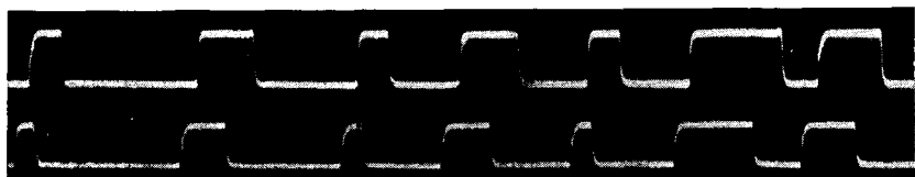
FIG. 16. Oscillograms of distorted telegraph signals (below) and the regenerated signal (above). (Reference 26.)
