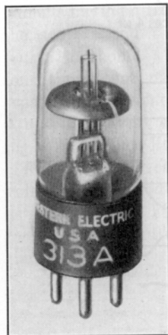
FIG. 8. A three-electrode cold-cathode gas-filled tube of the general type sometimes used in selective-ringing circuits as explained on page 358. (Courtesy Western Electric Co.)
